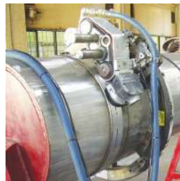
Installed machine performing overlay sanding operation
